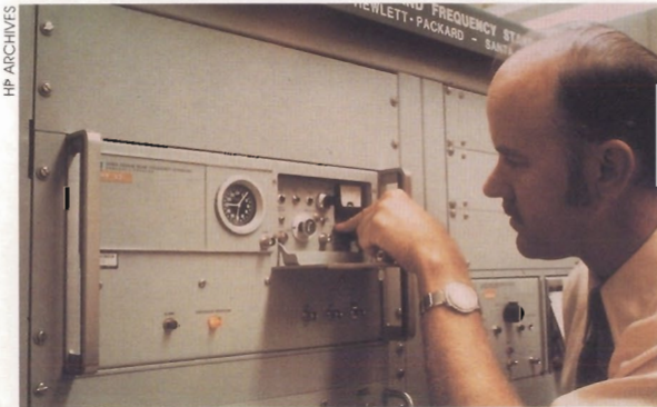
Hewlett-Packard gained worldwide recognition in 1964 when two HP 5060A "atomic clocks" coordinated the national time standards of various countries to within a millionth of a second.
