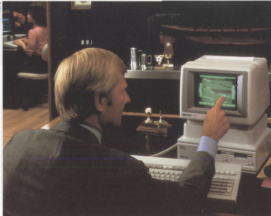
The HP Touchscreen personal computer—the HP 150—presented a new concept in hands-on computing when it reached the market in 1983.
